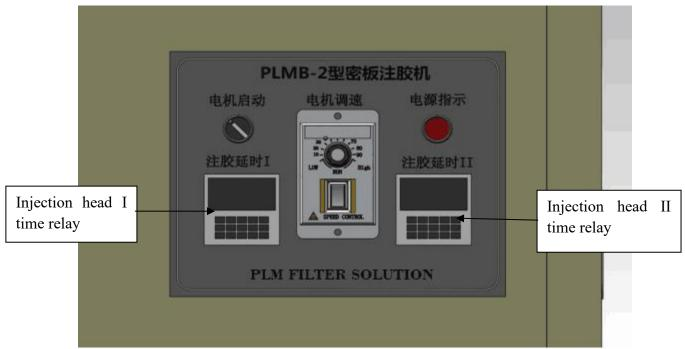
2.4 Adjustment of injection volume of injection head:
